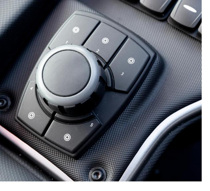
The new and exclusive touchscreen facilitates access to all the vehicle controls. Also, it includes a joystick on the left side of the driver's seat which allows to control all the functions in the screen in a safe way, avoiding potential driving distractions.
